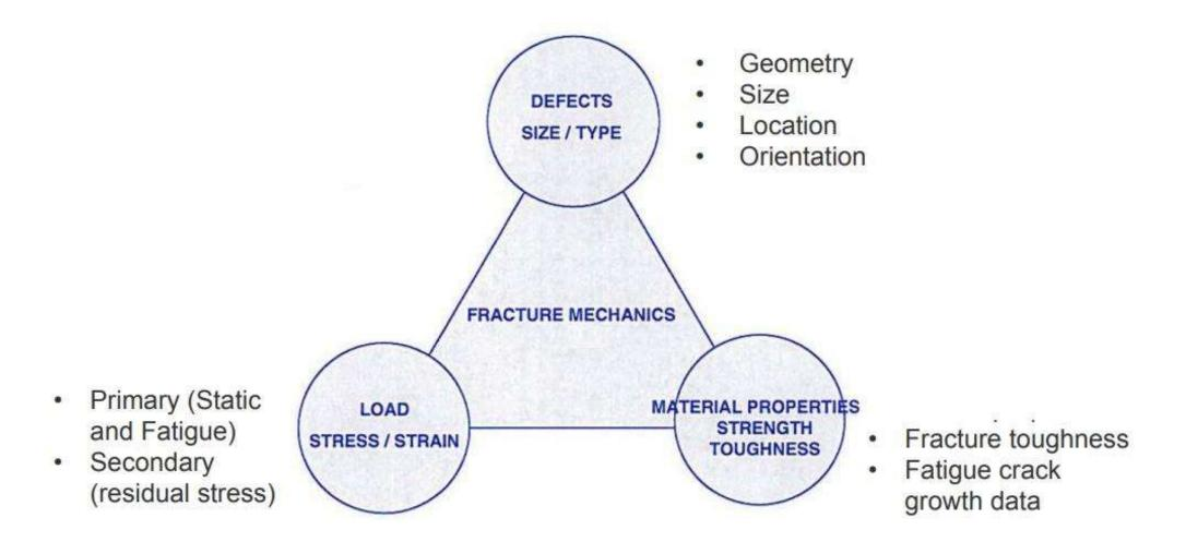
$$K = \sigma Y \sqrt{\pi a} \qquad \Delta K = \Delta \sigma \cdot Y \cdot \sqrt{\pi a}$$
